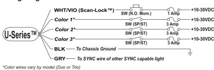
NOTE: All wires are 22 AWG. All switches and fuses are customer supplied.
